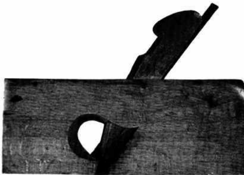
Figure 25. 1830–1840: THE DESIGN of the rabbet plane, used to cut a groove of fixed width and depth on the edge of a board, was not improved upon in the 19th century. The carpenter's dependence on this tool lessened only after the perfection of multipurpose metallic planes that could be readily converted to cut a "rabbet." (Private collection. Smithsonian photo 494789-)
