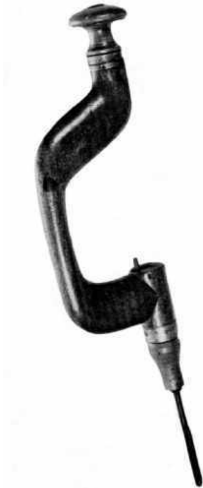
Figure 46.—18 TH CENTURY: THE BRACE AND BIT in its nonfactory form conforms to a general design pattern in which none of the components are ever precisely alike. This aspect of variety of detail—sophistication, crudeness, decorative qualities or the like—reflects something of the individuality of the toolmaker, a quality completely lost in the standardization of the carpenter's brace. (Smithsonian photo 49794-A.)
