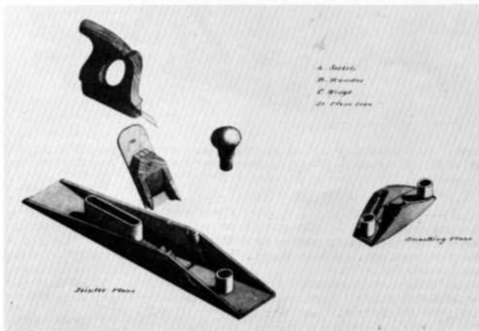
Figure 58.—1827: THE BENCH PLANES exhibited at Philadelphia in 1876 were a radical departure from the traditional. In 1827 H. Knowles patented an iron-bodied bench plane that portended a change in form that would witness a substitution of steel for wood in all critical areas of the tool's construction, and easy adjustment of the cutting edge by a setscrew, and an increased flexibility that allowed one plane to be used for several purposes. (Wash drawing from the restored patent drawings, August 24, 1827, U.S. Patent Office, Record Group 241, the National Archives.)
