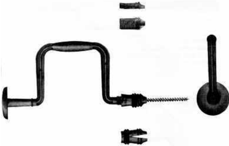
Figure 44.—1865: MILTON NOBLES' PATENT perfecting the chuck which held the auger bit was an important step along the path which led ultimately to the complete acceptance of the metallic brace. Barber's ratchet brace shown in figure 66 completes the metamorphosis of this tool form in the United States. (Original patent drawing 51,660, U.S. Patent Office, Record Group 241, the National Archives.)
