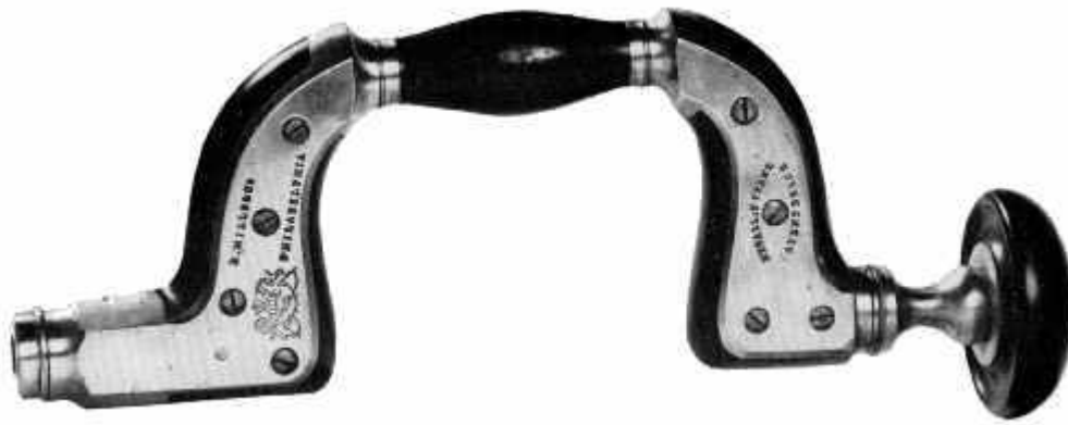
Figure 57.—1876: JAPANNED AND SPLINTED WITH HEAVY BRASS, this brace was among the award-winning tools exhibited at the Centennial by E. Mills and Company of Philadelphia. (Smithsonian photo 49792-D.)
