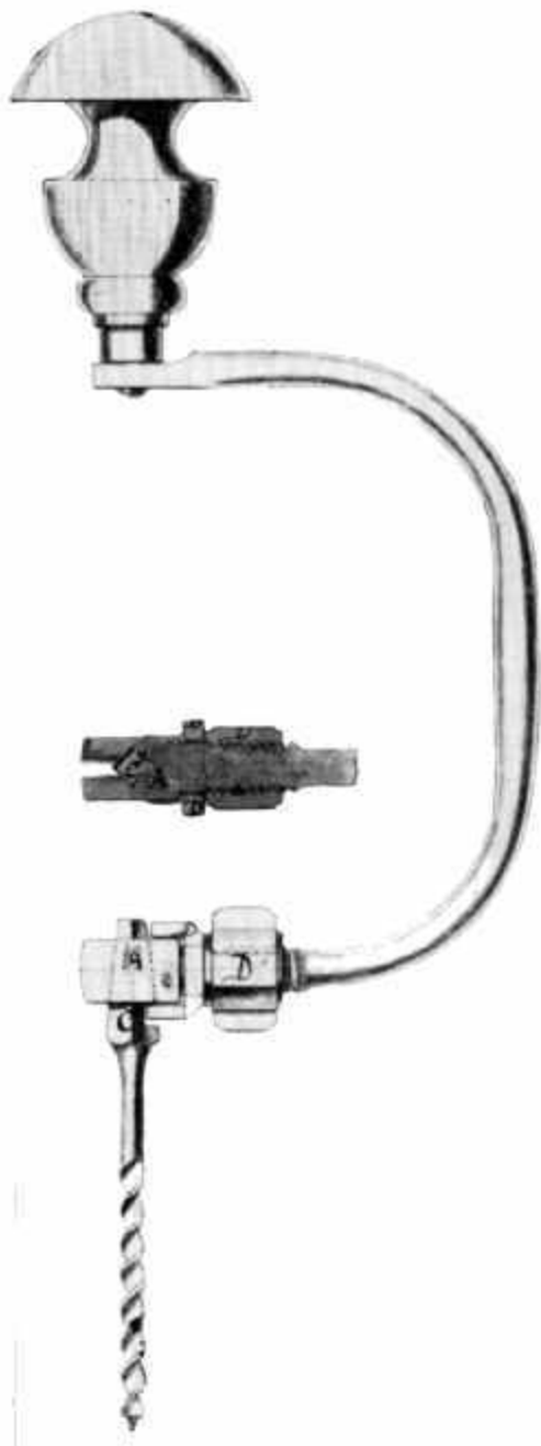
Figure 43.—1866: THE SIMPLICITY AND STRENGTH of the brace proposed by J. Parker Gordon is in sharp contrast to the heavily splinted sides of the wooden brace commonly used in mid-19th-century America. (Original patent drawing 52,042, U.S. Patent Office, Record Group 241, the National Archives.)
