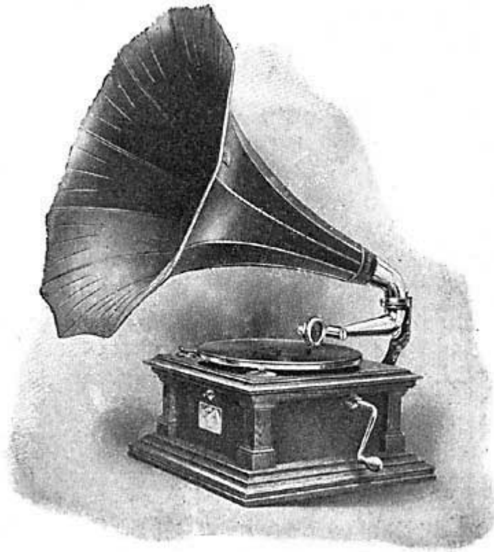
FIG. 196.—A phonograph. In this machine the cylinder is replaced by a revolving disk.
