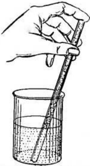
FIG. 42.—Water rises in the tube when the air is withdrawn.
