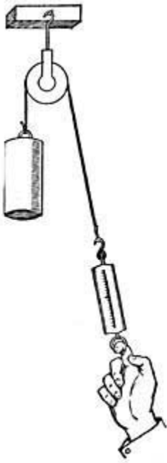
FIG. 109.—By means of a pulley, a force in one direction produces motion in the opposite direction.
