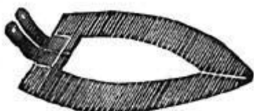
FIG. 202.—The fine wires are strongly heated by the current which flows through them.
