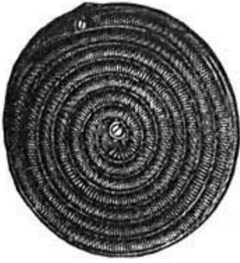
FIG. 205.—The heating element in the electric stove.
