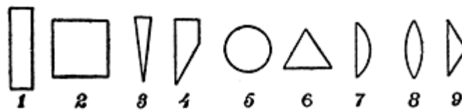
Fig. 54. Cross Sections of Files. ToList
