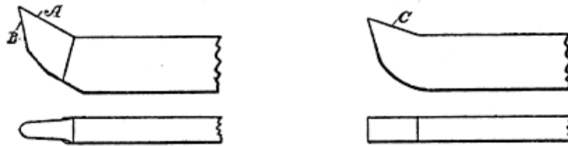
Fig. 24. Tool for Wrought Iron. Fig. 25. Tool for Cast Iron. ToList
