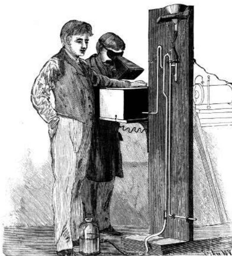
FIG. 217.—EDISON'S SURGEON'S X-RAY APPARATUS.
