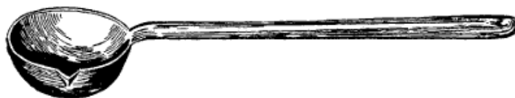
Figure 98.—Melting Ladle. Babbitting shaft boxings requires a melting ladle. It should be about five inches across the bowl and about three inches deep. That is a good size to heat in a forge fire.
