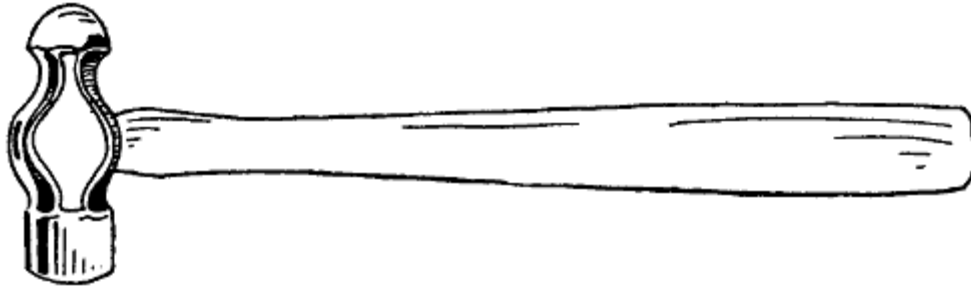
Figure 55.—Machinist's Hammers. A medium weight should be selected for farm repair work. It should be hung so the end of the handle clears half an inch when the face rests flat on the bench.
