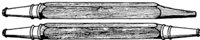
Figure 72.—Wooden Wagon Axles. Axle timber may be bought in the rough or partly fitted to the skeins.
