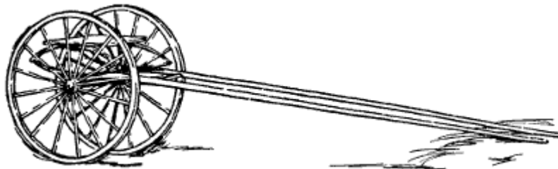
Figure 169.—Colt-Breaking Sulky. The axle and hind wheels of a light wagon, two strong straight-grained shafts about 4 feet too long, a whiffletree and a spring seat are the principal parts of a colt-breaking sulky. The shafts and seat are thoroughly well bolted and clipped to the axle and braced against all possible maneuvers of the colt. The traces are made so long that the colt cannot reach anything to kick, and he is prevented from kicking by a strap reaching from one shaft up over his hips and down to the other shaft. In this rig the colt is compelled to go ahead because he cannot turn around. The axle should be longer than standard to prevent upsetting when the colt turns a corner at high speed.
