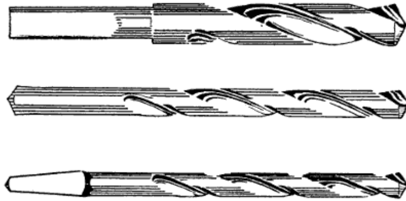
Figure 51.—Twist-Drills. Round shank for the post drill and square taper shank for brace work. Brace drills are small, \frac{1}{4} " or less.
