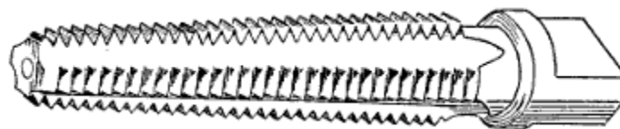
Figure 84.—Taper Tap for Blacksmith's Use.
