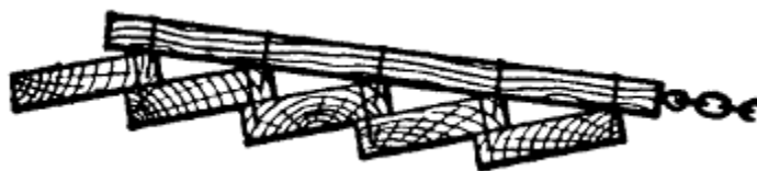
Figure 140.—Land Float. Clod crushers and land floats belong to the same tribe. Theoretically they are all outlaws, but some practical farmers harbor one or more of them. Wet land, containing considerable clay, sometimes forms into lumps which should be crushed.
