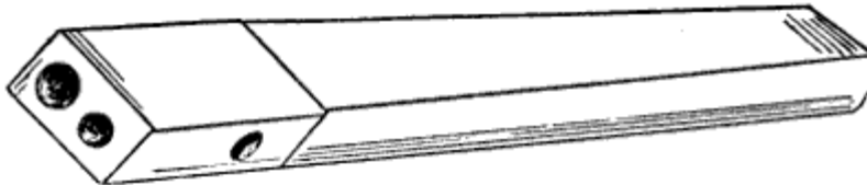
Figure 78.—Rivet Set. This style of set is used for small rivets. The size should be selected to fit the rivets closely. Larger rivets are made to hug the work by means of a flat piece of steel with a hole through it.
