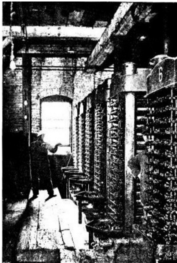
Photo by Press Illustrating Service Cottonseed Oil As It Is Squeezed From The Seed By The Presses
