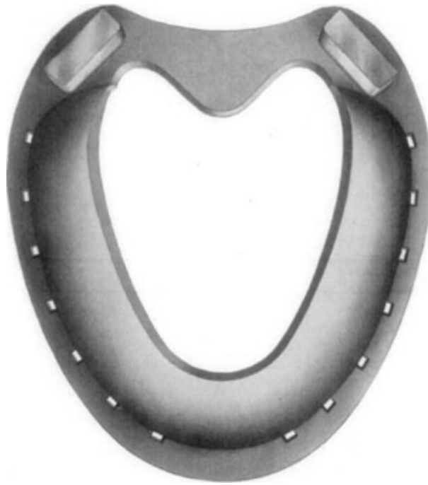
Fig. 35—Inferior (convex) surface of Cochran shoe.
