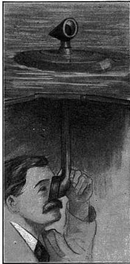
FIG. 102—HOW MEN IN A SUBMARINE SEE WHEN UNDER THE WATER
